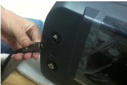
4.3 Connect well the foot switch to Device.
